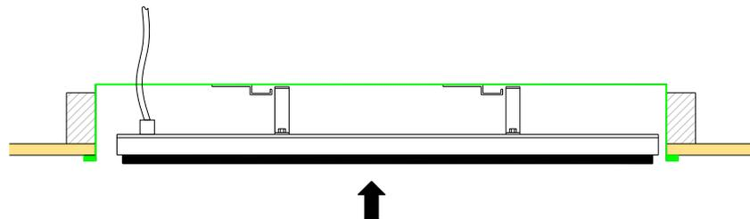
**STEP 5:** Push the heater to the left ensuring the brackets engage in the mounts. It will then drop in. Shake the heater to ensure that it is securely mounted.
