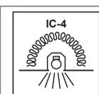
Recessed Luminaire where fixed building insulation material can abut and cover the recessed luminaire. Building Insulation does not have to be non flammable. Building Insulation must maintain structural integrity at 90 degrees C.
